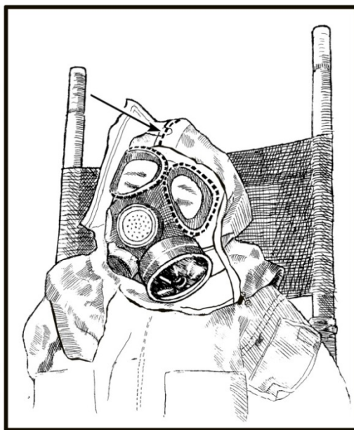
Figure 5-3. Cutline for hoods integral to overgarments
