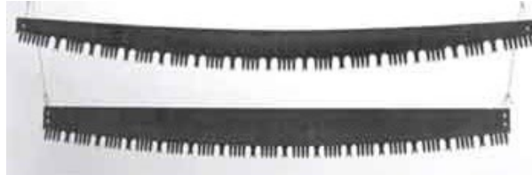
Comparison of felling and bucking saws.
